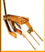
Double Shoe -The Double Shoe will plant the seeds in Two Lines--2" apart. It is only used with the 24 hole roller -- The divider will drop the seed down each side thus creating 2 lines of 12 holes.
